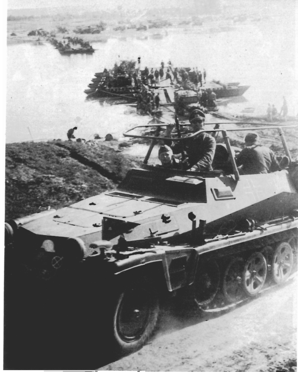
As can be seen in this picture; this is a light SPW (250/3) of the "Grossdeutschland" Panzer-Grenadier Division. This one is a command car (note the emblem at left front) of the "GD" Motorcycle Rifle Battalion (as shown by the divisional and tactical emblems on the bow of the vehicle).
