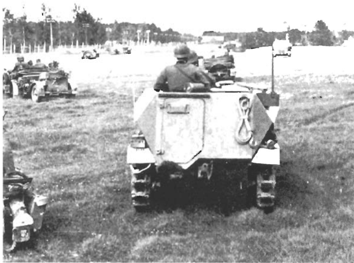
A light armored observation car (Sd.Kfz.253), also based on the 250 type. They were to be found in the artillery units within the Panzer divisions.
