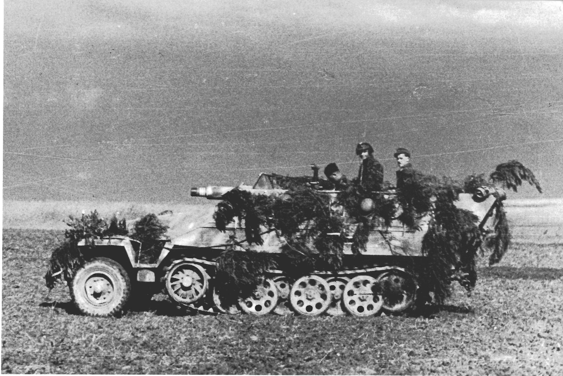
After Kampfpanzer IV and Sturmgeschütz III were fitted with longer guns, the remaining KwK and Stuk guns were installed in Schützenpanzerwagen. (2 x BA)
