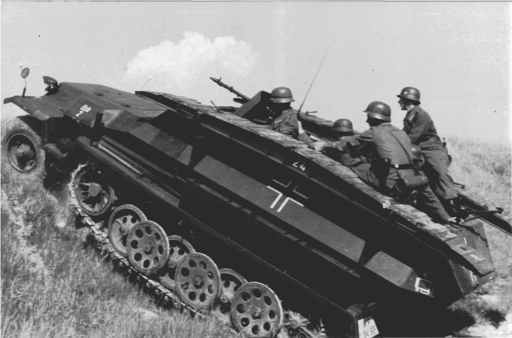
The medium Pionier-Geräte-Schützenpanzerwagen, Sd.Kfz.251/7, seen on this page as Type C and on the right page as Type D. Both photos show them with assault bridges; they also existed without them. (1 x BA)
